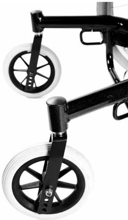
Rotate the front wheels of the Leckey Tour Mobility Base so that they are in a forward facing direction in order to improve stability of the unit (Fig 21).
