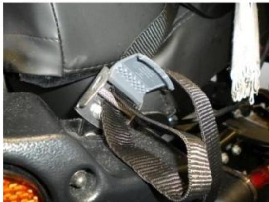
The Leeway was retro-fitted to Neil's chair cushion using a simple Velcro strap and secured to the frame using existing cinch mounts and triglides.
